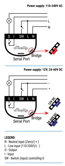
The WiFi Relay Switch Shelly 1 may control an electrical circuit up to 3.5 kW. It is intended to be mounted into a standard in-wall console, behind power sockets and light switches or other places with limited space. Shelly may work as a standalone Device or as an accessory to a home automation controller.
